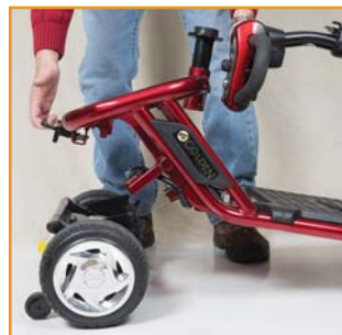
While squeezing the release lever, pull up on the rear frame
