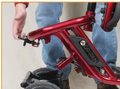
To separate the rear transaxle from the frame, squeeze the release lever located on the underside of the frame
